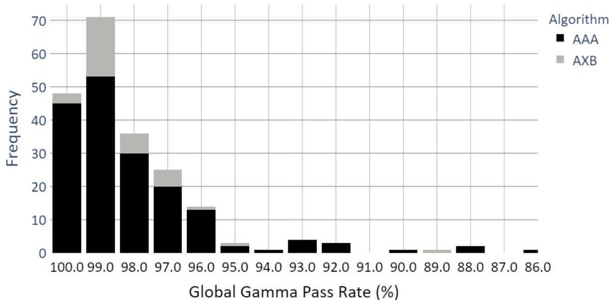
Figure 7: Global gamma pass rate (3%/3mm, 10% max dose threshold) for VMAT plans on conventional linacs for AAA (black) (n=176) and AXB (grey) (n=35). A single gamma value of 71.3% for
