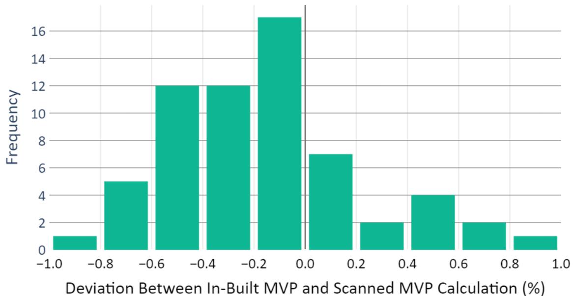
**Figure 3** Histogram showing the difference between a M3D calculation reported mean dose to the ionisation chamber between the in-built MVP (excluding couch) and from the locally CT scanned MVP (including couch) (n=63). A negative deviation shows the locally scanned MVP reporting a lower dose.
