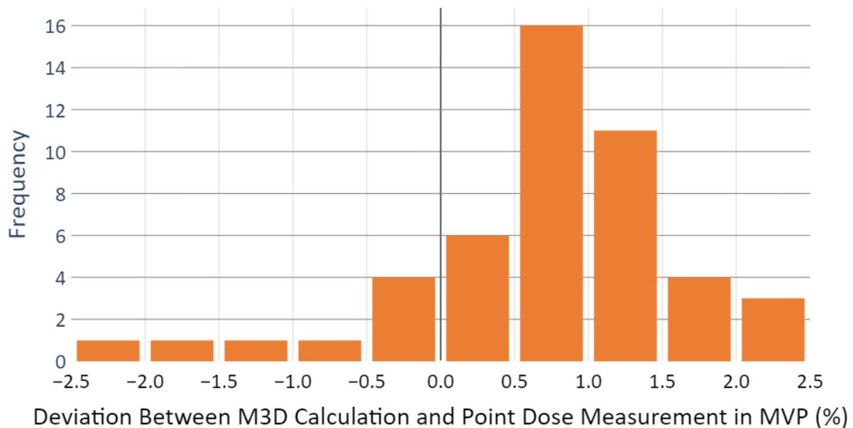
**Figure 4** Histogram showing the difference in the MVP between a M3D calculation reported mean dose to the ionisation chamber and the dose physically measured at that point (n=48). A positive deviation shows the M3D calculation reporting a higher dose.
