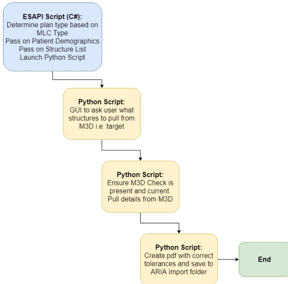
**Figure 10 Top Level view of ESAPI and Python Script Logic Flow**
