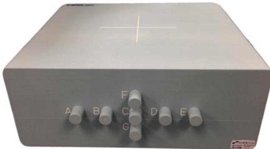
**Figure 2: Mobius Verification Phantom with seven measurement points and a slice for holding film. Manufactured from water equivalent material.**
