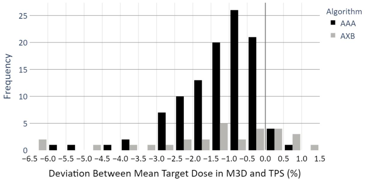
Figure 6 Histogram showing the difference in the mean target dose between the M3D calculation and the TPS dose for VMAT plans for two algorithms: AAA (black) (n=108) and AXB (Dose to Medium) (grey) (n=28). A negative deviation shows the M3D calculation reporting a lower dose than the TPS.
