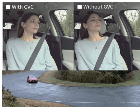
* In-house passenger seat comparison of left-hand turn at 30 km/h (lateral acceleration of 0.4 G)
