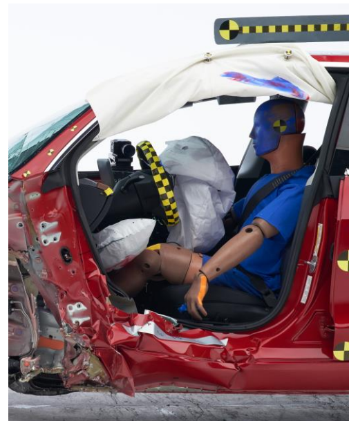
The 2019 Model 3 generally held up well in the driver-side small overlap front test. However, the lower door-hinge pillar moved in 8 inches, and the door sill buckled.
