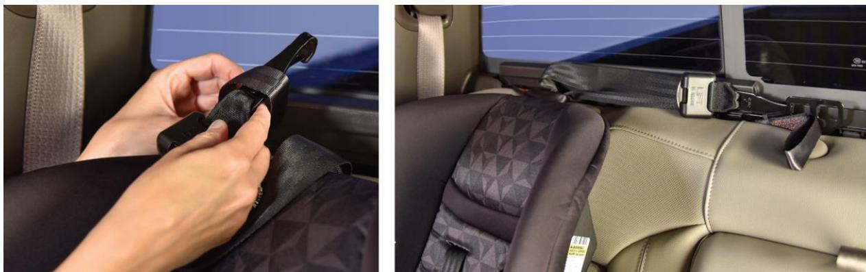
**Pickups like this one (shown with head restraints removed) typically require child seat tethers to be fed through a loop at the top of the vehicle seat (left) and then attached to a loop or anchor above an adjacent seating position. This complexity makes it hard for pickups to earn good LATCH ratings.**
