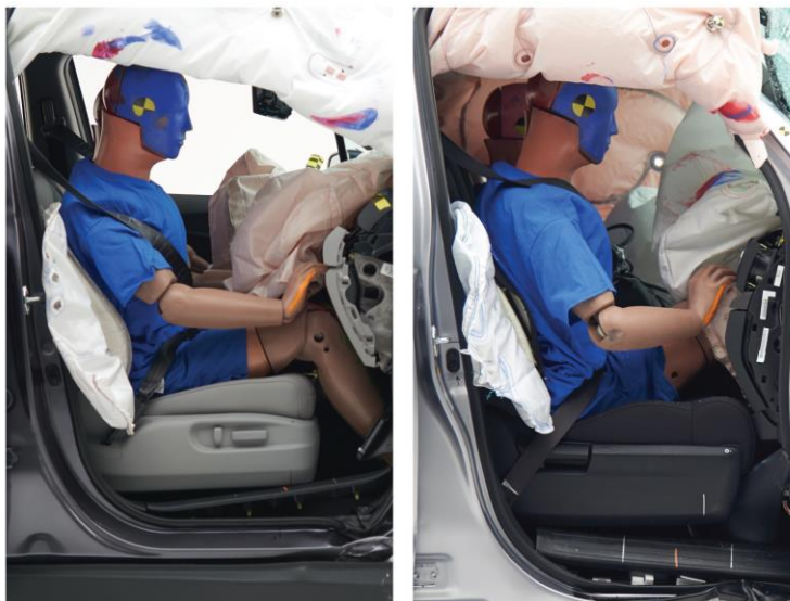
The structure of the Honda Ridgeline (left) held up well, while the Toyota Tundra had severe intrusion into the passenger space.
