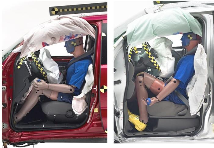
**In the Toyota Tacoma Double Cab small overlap test (left), the dummy's position in relation to the door frame, steering wheel and instrument panel indicates that the driver's survival space was well-maintained. In contrast, the structure of the Nissan Frontier Crew Cab (right) allowed too much intrusion into the occupant compartment, compromising driver survival space.**
