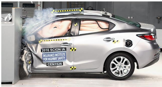
**The Scion iA is rated good in the small overlap front test and is the first low-priced model with standard autobrake.**
