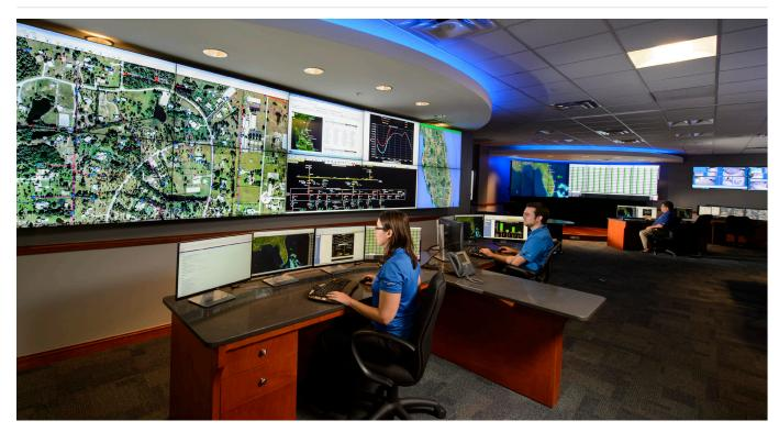
FPL leverages smart grid technology and predictive analytics to deliver real-time data to engineers in the diagnostic center. FPL engineers analyze the data to measure and improve the health and performance of the grid and deliver better, more efficient electric service to customers.
